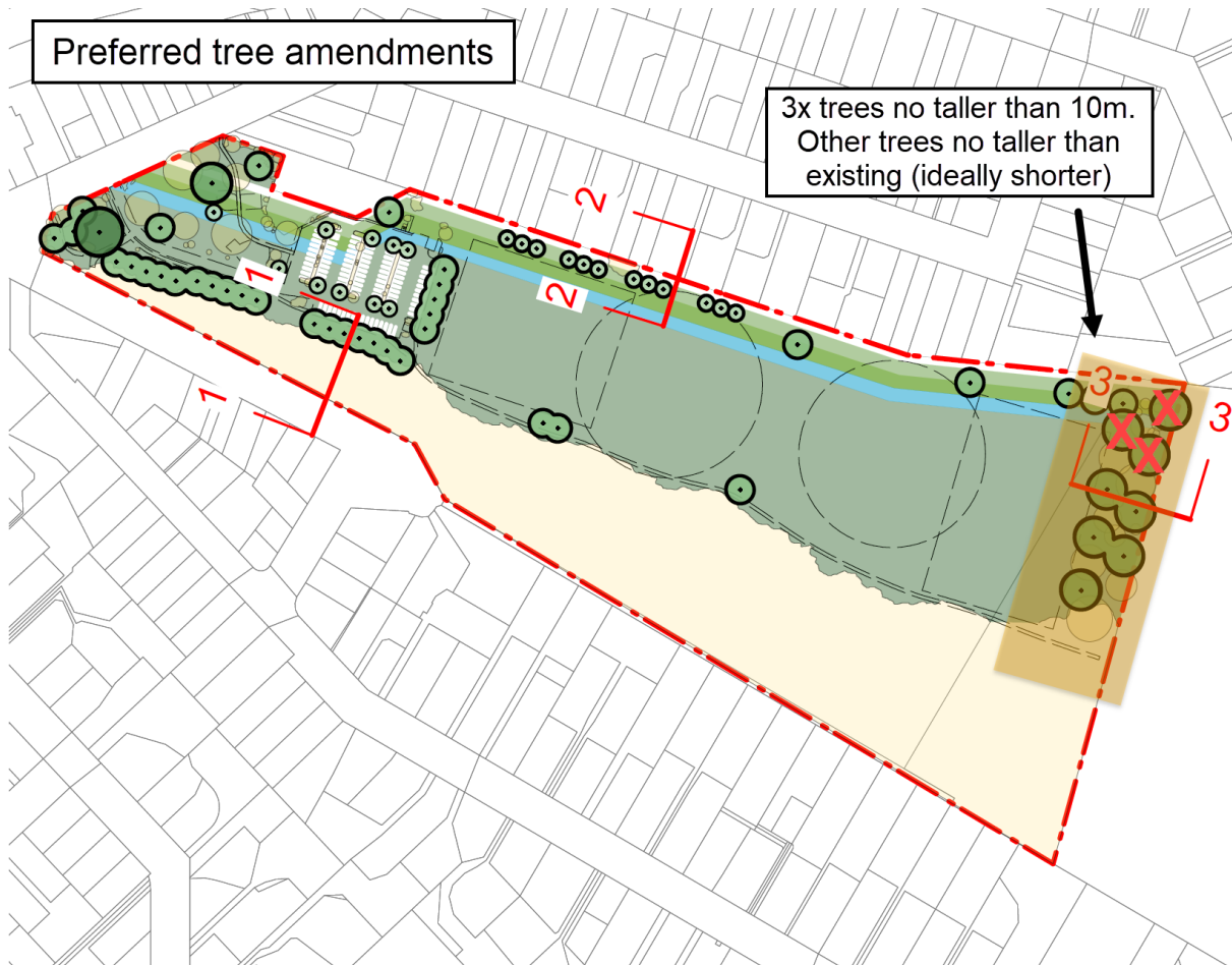
Figure 1 : Cloudbase suggestion for planting at Barnett Park. X marks trees that cause issues for operation of the school
