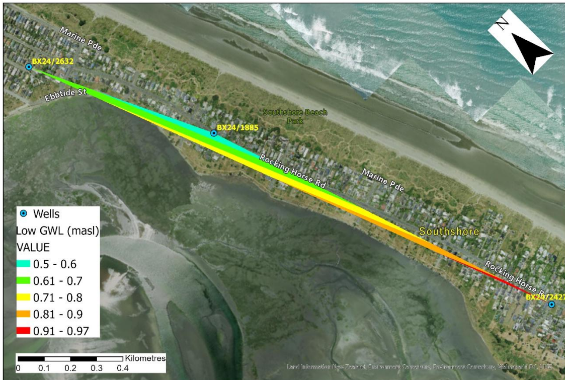
Figure 7: Map of the interpolated lowest groundwater levels (masl) during the representative low groundwater period in summer 2017-18. Note the groundwater flow direction being to the east, moving away from the estuary, which is likely contributing to the groundwater. The steeper gradient of the water levels shows a higher flow rate for the shallow groundwater.
