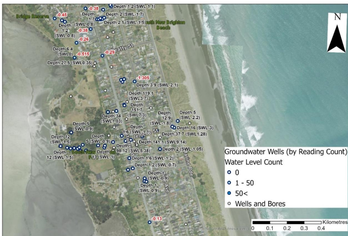
Figure 3. Map of the South Brighton Park area showing groundwater wells and wells classed by reading count. Note the lack of shallow continuous groundwater level wells around the park site, with most readings limited to periodic or the initial (Static) water level in the well when drilled (SWL). Many of the shallow SWL readings show the groundwater as less than 1m below ground level, with the shallowest showing 0.13m below ground level at well BX24/2292 towards the south of the map.
