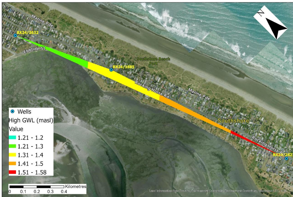
Figure 8: Map of the interpolated highest groundwater level (masl) from the selected shallow triangulating wells, during the representative high groundwater period in the winter of 2019. Note that the flow direction differs from the low groundwater period, with the groundwater flowing to Northwest and likely flowing to the estuary.
