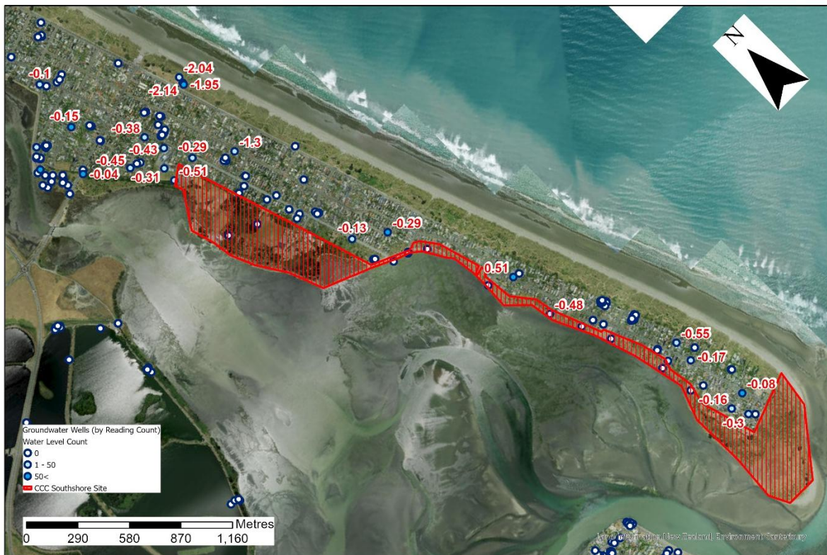
Figure 2: Map of the South New Brighton Park and Southshore area showing shallow (less than 10m) deep wells highest groundwater levels (from ground level) and the approximated area of proposed works. Note the very shallow groundwater levels across the area especially in the low-lying areas near the shoreline of the Avon-Heathcote Estuary, and the lack of shallow groundwater readings near the SNBP.
