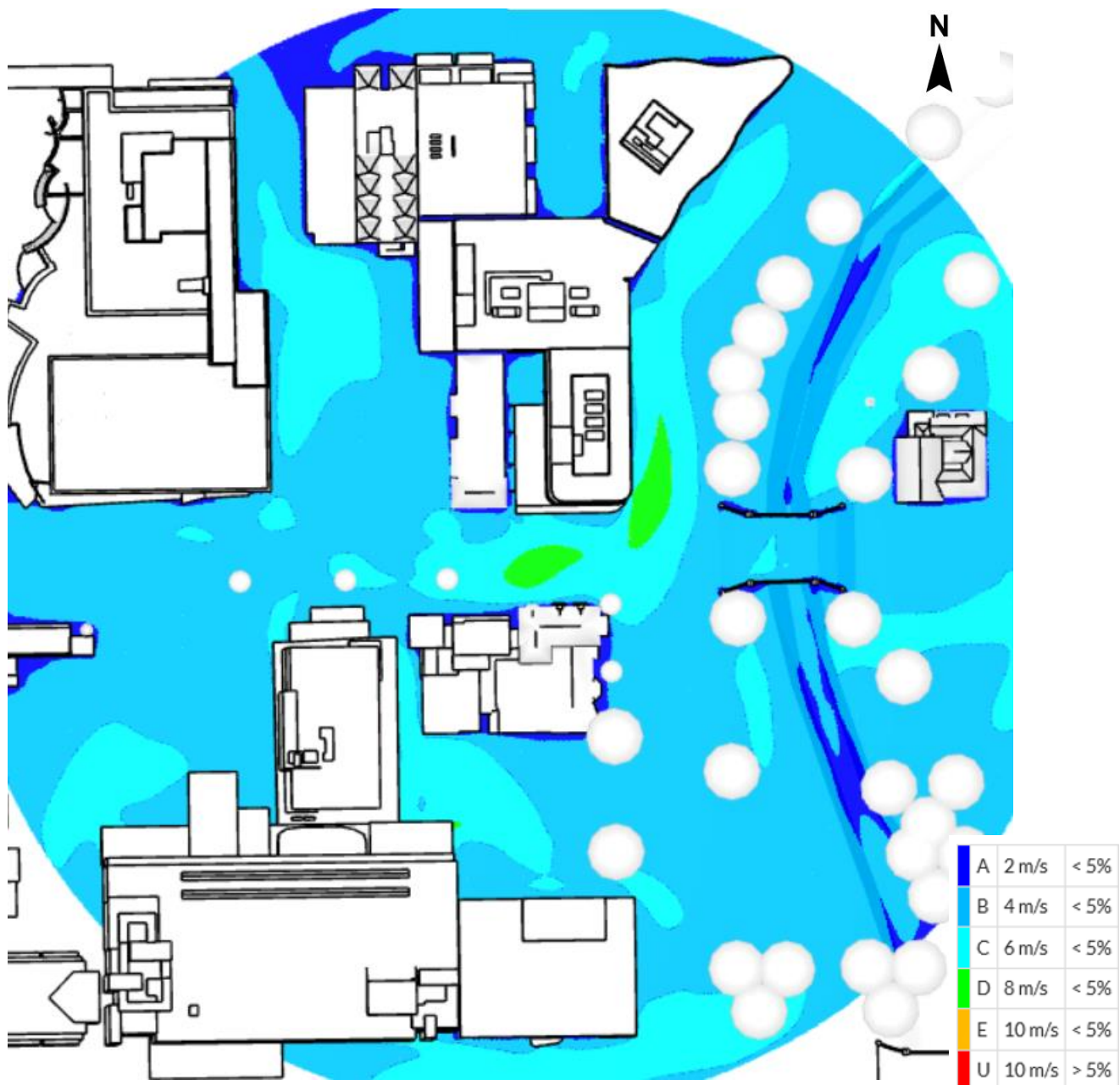
Figure 4: All sector pedestrian wind comfort with the proposed new building and Harley Chambers demolished - Lawson LDDC
