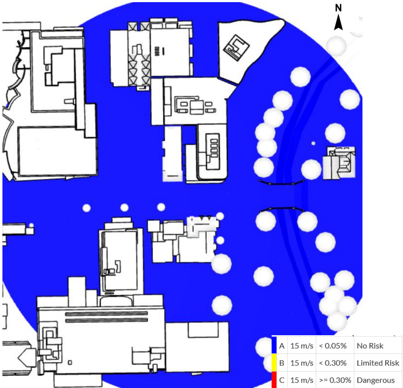
Figure 6: All sector pedestrian wind safety for new build scenario - - NEN 8100
