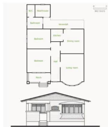
Floor plan and principal elevation of a typical bungalow. Te Ara The Encyclopedia of New Zealand .
