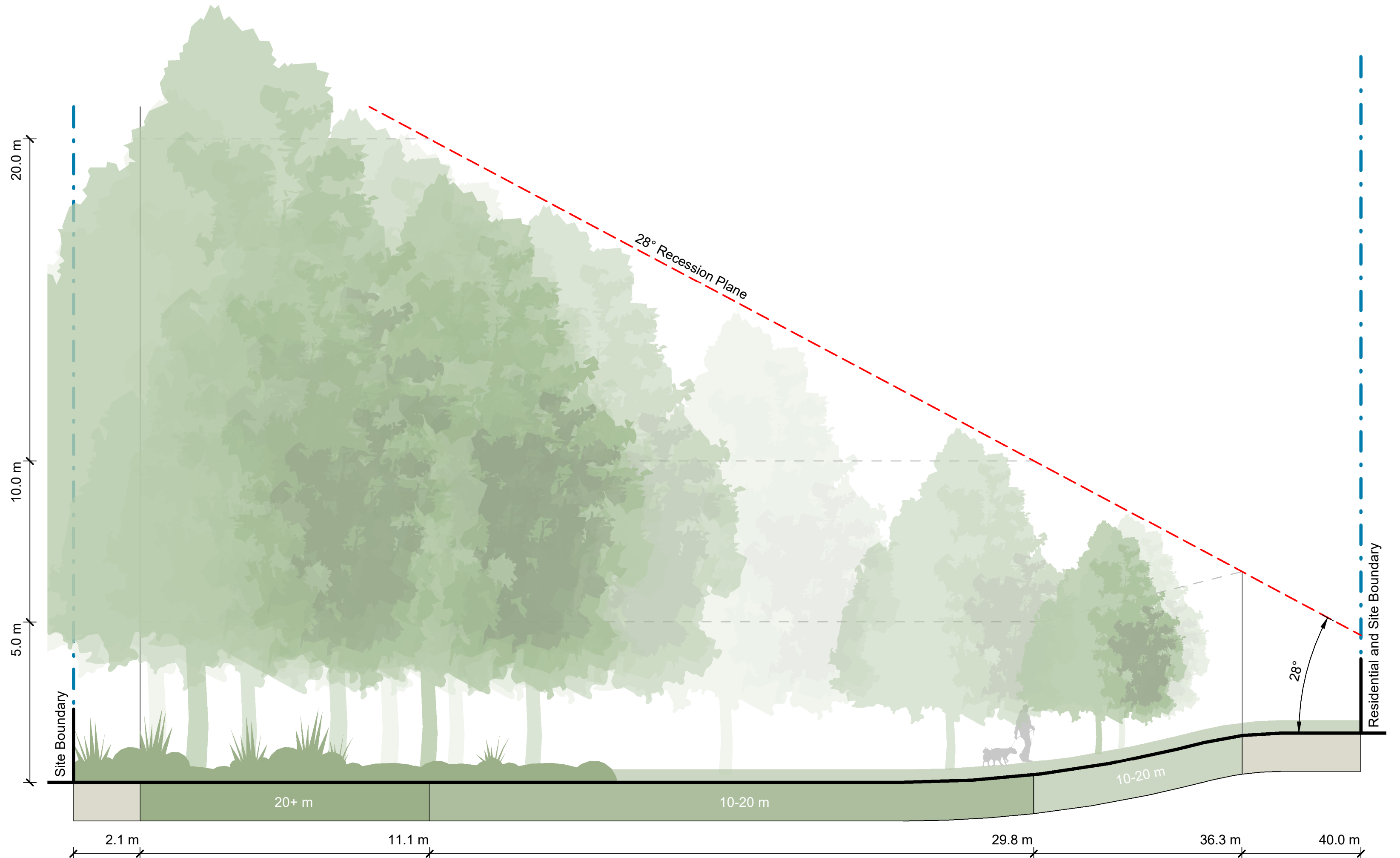
6 North-South Cross Section 2 - Heathcote Scale: 1 : 100
