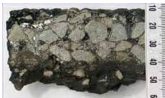
An example of aggregate bound by coal tar in a road surface.
