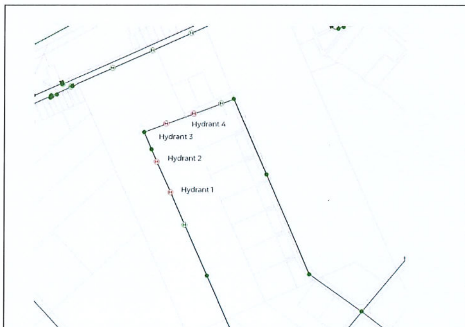
Figure 3-3 : Selected hydrants for FW4 fire flow criteria
