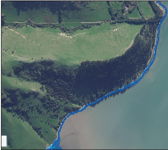
Figure 3: Section of Wharf Road unaffected by coastal flooding as it sits significantly above sea level.
