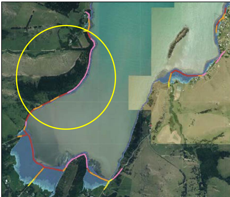
Figure 4: Wharf Road (left of bay), pink line that indicates area potentially prone to erosion that is the main vulnerability of Wharf Road, not sea level rise.
